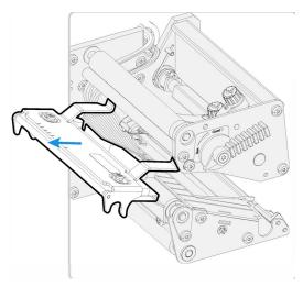
8. Disconnect the cables from the printhead. Note the snap-lock on the inner connector. Pull at the connectors, not at the cables.
