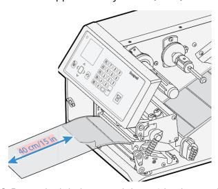
12. Route the labels around the guide plate and back under the print unit to the take-up hub.
