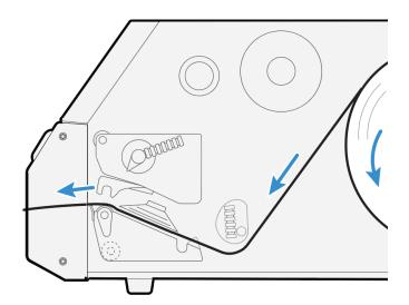
14. Turn the printhead lift lever clockwise to lower the printhead.
