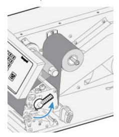
4. Remove any empty core from the media supply hub.
