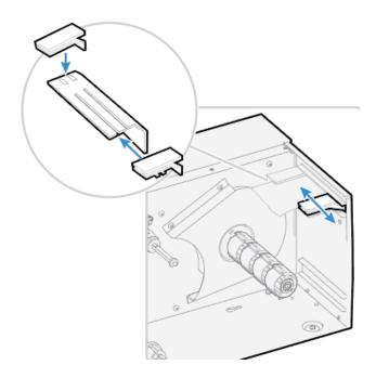
2. Feed the media through the slot in the rear plate.
