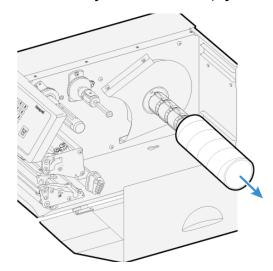
6. If you are using a media roll with a 76 mm (3 in) core, install a 3-inch adapter on the media supply hub.
