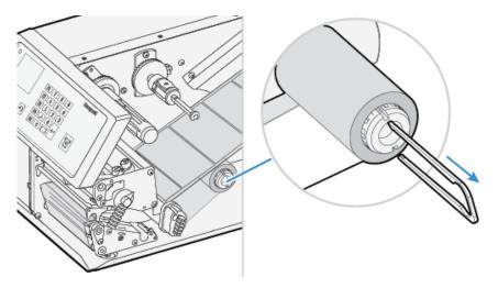
6. Remove any empty core from the media supply hub.
