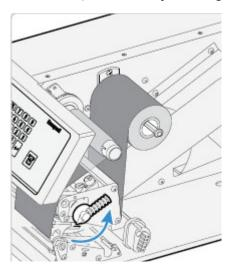
5. Pull out the green clip on the liner take-up hub and dispose of any wound-up liner.
