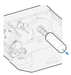
7. If your are using a media roll with a 76 mm (3 in) core, fit an adapter on the media supply hub.
