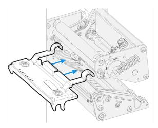
10. Connect the hooks of the printhead bracket to the headlift shaft. Make sure that the cables are not in the way.
