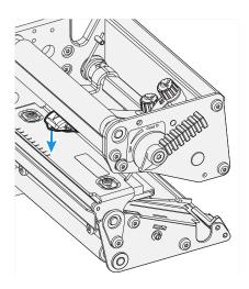
7. Disconnect the hooks of the printhead bracket from the shaft and pull out the printhead as far as the cables allow.
