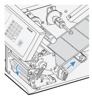
13. Secure the liner to the take-up hub with the green clip and rotate the hub until the media is pulled tight.
