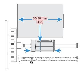
• If your ribbon is 110 mm (4.3 in) wide, compress the ribbon supply bobbin and move it so it snaps into the third (outermost) groove.
