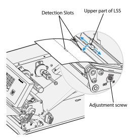
2. Look at the print mechanism from the front with the printhead lifted to make sure that the point of detection on the upper sensor is aligned with the center of the slots or marks in the media.
