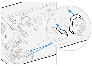
13. Close the front door and media cover. Make sure that the media runs through the slot in the front door.
