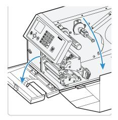
2. Pull the upper guide straight out and press the snap-lock, lift the edge of the lower guide, and pull the lower guide straight out.
