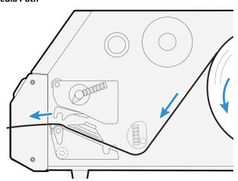
10. Turn the printhead lift lever clockwise to lower the printhead.
