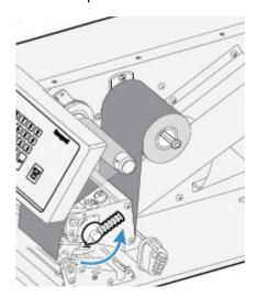
5. Remove any empty core from the media supply hub.
